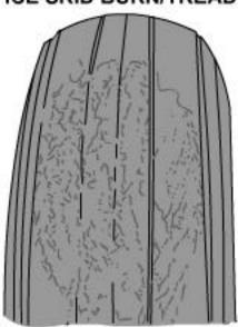
Tyres with ice burns/tread rubber reversion are not servicable if the damage exposes the tread reinforcement or cut protector plies or tyre balance is affected
