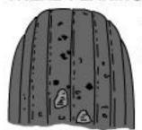
Tyres with flaking, chipping or chunking are not servicable if any fabric is exposed
