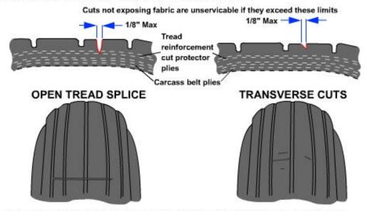
Tyres with an open splice are not servicable. A closed tread splice will appear as a thin line crossing the tread ribs Transverse cuts contained within a rib and penetrating into the carcass plies (bias) belt plies (radial) are not servicable. Cuts extending across a rib from groove to groovethat are deeper than the groove are not servicable
