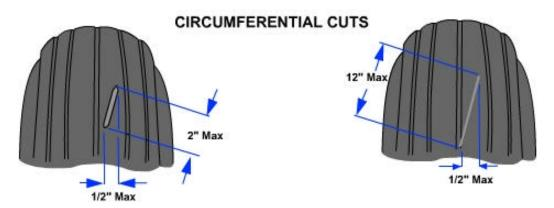
Cuts penetrating the tread reinforcement / cut protector plies are not serviceable if cut penetrates the carcass plies (bias) or belt plies, (radial), cut is not contained in one rib
